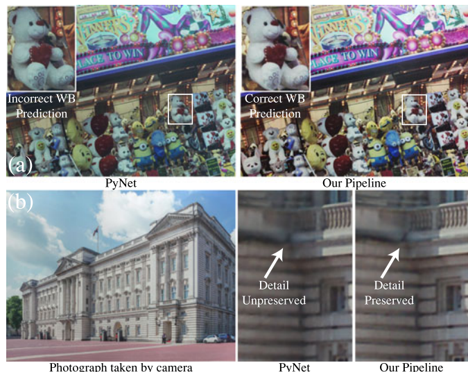
Fig. 11. Comparisons with the deep-learning ISP. (a) the failure case of the deep-learning ISP in white balance prediction. (b) evaluation on the ability of detail preservation.
