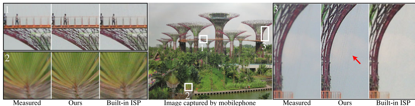
Fig. 10. Comparisons with built-in ISP. Note that the built-in ISP smooths out the cords, yet our method restores it (marked with the red arrow).
