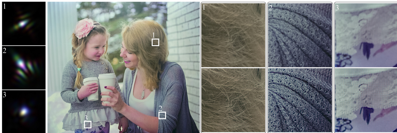
Fig. 1. We present a practical method for optical aberrations correction. We calculate the spatially variant PSFs (shown on the left in 10 \times resampling) of a specific lens by the proposed optical PSF model (Section 4). The PSFs are used for imaging simulation to generate training data for the proposed postprocessing chain (Section 5). Our approach significantly improves image quality (shown on the right) and is convenient for deploying to new devices.
